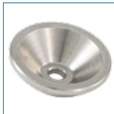
The outside of the adapter is spherical with Ø1.5". After inserting the Ø30 mm ball on the conical inner part, the ball centre (= visible prism centre) is at the same height as the centre of a directly inserted Ø1.5" ball. On stainless steel bases the height is therefore 25 mm (see picture 1) and on blue bases 38.1 mm (see picture 2).
