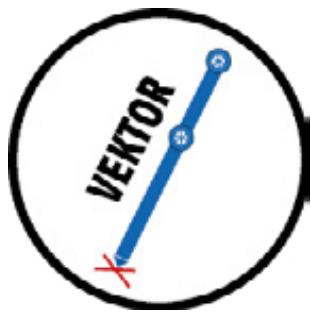
For the measurement of hidden points (mathematical extension of a base where 2 prisms are measured tachymetrically according to X, Y and Z).
