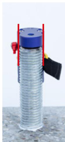
The BOAXE consists of a 90° attachment prism and a screwed-on „lid“ as upper part. These must be combined depending on the diameter of the bolt.
