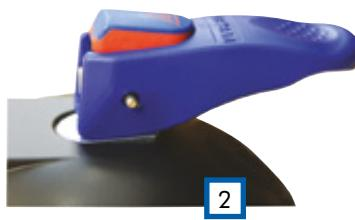
The vacuum is continuously checked. If the warning rocker switch is recessed in the rocker arm (see Fig. 1), the required holding force has been achieved and the suction cup can be fully loaded. If the rocker over time moves out and the red edge becomes visible, the vacuum decreases. If the edge is clearly visible (see Fig. 2), the suction holder must be detached from the surface and sucked on again.
