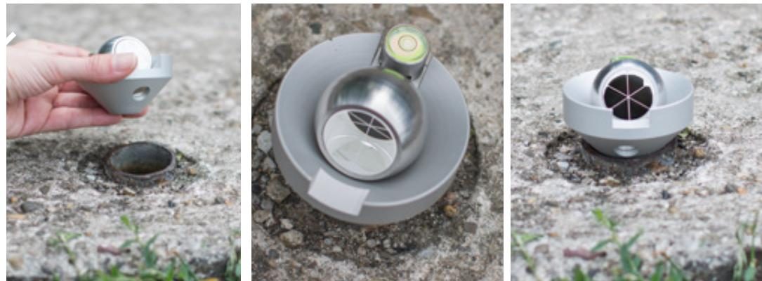
In the example shown here, the axis pin has been left out, since the ball prism can also be inserted without the cone adapter axis pin.
