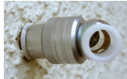
For ball prisms Ø1.5" with glass-Ø25 mm
