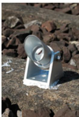
■ Screwed directly to the object with the 4 eccentric boreholes Ø 5 mm
