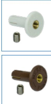
Wall bolt made of plastic with continuous brass core, which is spread by a threaded pin. Inscription „Messpunkt“. For spreading of the shaft an Allen key is required.
