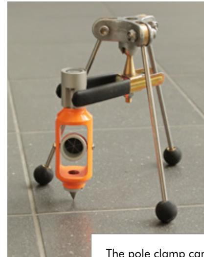
The pole clamp can be aligned downwards for lower positions.
