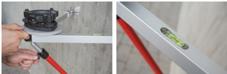
Fixing the ball joint of the telescopic arm
